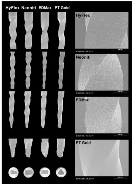
**FIGURE 2** SEM analyses of the active blade, cross-section design, tip geometry, and surface finishing of tested instruments. All instruments had asymmetrical blades, no radial lands, and different cross-section designs and tip geometries. HyFlex EDM, Neoniti and EDMax instruments had isotropic surface with regularly distributed crater, while ProTaper Gold had parallel gridding marks.
