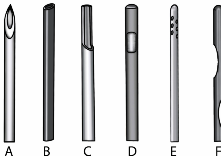
Fig. 1. Representation of endodontic needle types. Open-ended (A) beveled, (B) flat, and (C) notched. Closed-ended (D) side-vented, (E) with multiple exits, (F) double side-vented.
